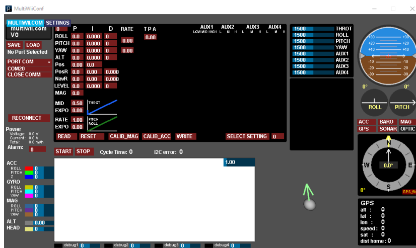
Figure 4 - Multiwii GUI - Screenshot of the interface for configuring an Arduino-based drone with MultiWii firmware. Photo credit: Miloš Rašić.
